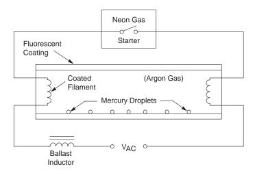
The above Figure illustrates a fluorescent lamp with the conventional glow–tube starter. The glow–tube starter consists of a bimetallic switch placed in series with the tube filament which closes to energize the filaments and then opens to interrupt the current flowing through the ballast inductor, thereby, generating the high voltage pulse necessary for starting. The mechanical glow–tube starter is the circuit component most likely to cause unreliable starting.
