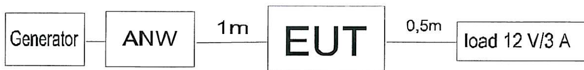
Fig. 1 Arrangement of tested equipment
