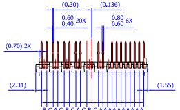
LEAD PITCH (TOLERANCE: ±0.30)
