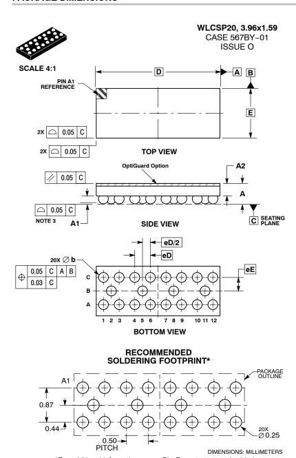
\*For additional information on our Pb-Free strategy and soldering details, please download the ON Semiconductor Soldering and Mounting Techniques Reference Manual, SOLDERRM/D.
