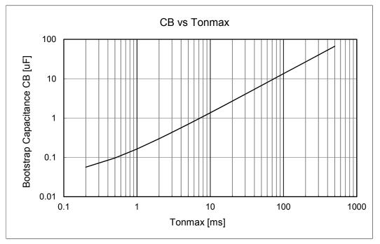
Fig. 12 Tonmax - CB characteristic
