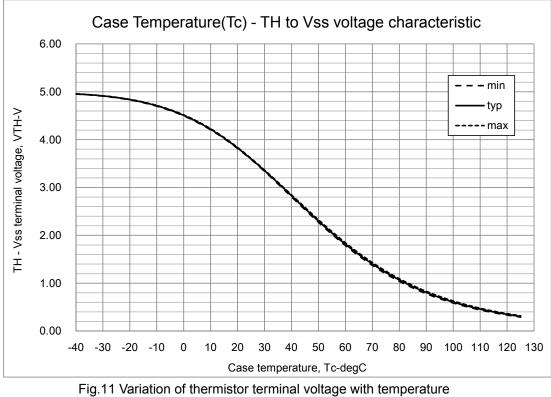
(39 k $\Omega$  pull-up resistor, 5 V)
