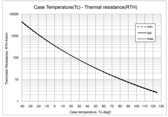
Fig.10 Variation of thermistor resistance with temperature
