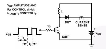
FIGURE 8.  $t_{rr}$  TEST CIRCUIT
