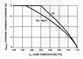
FIGURE 6. CURRENT DERATING CURVE
