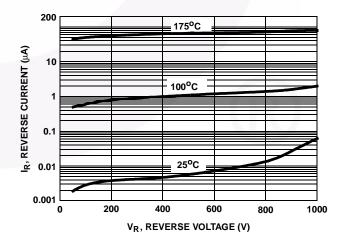
FIGURE 2. REVERSE CURRENT vs REVERSE VOLTAGE
