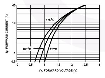
FIGURE 1. FORWARD CURRENT vs FORWARD VOLTAGE
