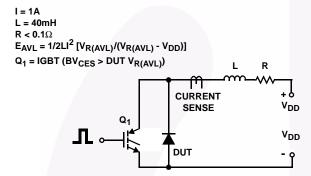
FIGURE 10. AVALANCHE ENERGY TEST CIRCUIT
