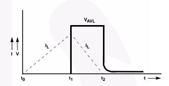
FIGURE 11. AVALANCHE CURRENT AND VOLTAGE WAVEFORMS
