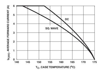
FIGURE 6. CURRENT DERATING CURVE
