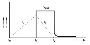
FIGURE 11. AVALANCHE CURRENT AND VOLTAGE WAVEFORMS
