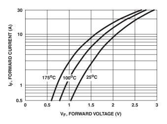
FIGURE 1. FORWARD CURRENT vs FORWARD VOLTAGE
