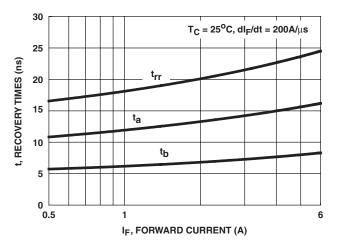
FIGURE 3. t<sub>rr</sub>, t<sub>a</sub> AND t<sub>b</sub> CURVES vs FORWARD CURRENT
