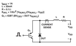
FIGURE 10. AVALANCHE ENERGY TEST CIRCUIT
