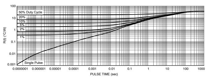
Figure 13. Transient Thermal Impedance
