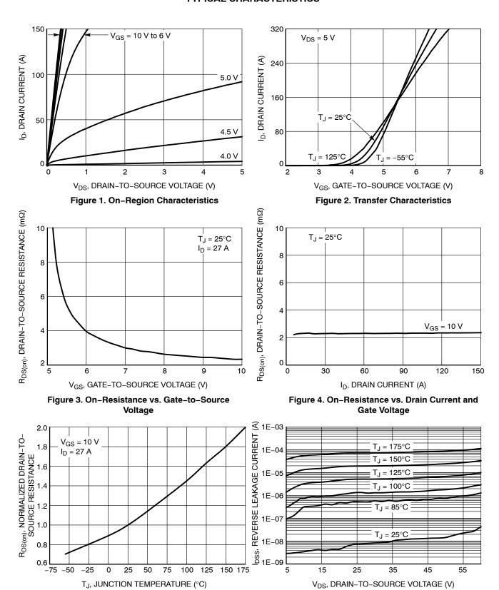
Figure 5. On–Resistance Variation with Temperature
