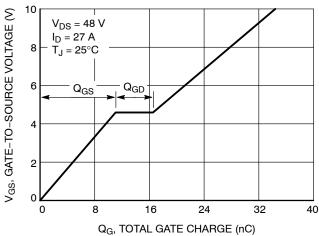
Figure 8. Gate-to-Source vs. Total Charge
