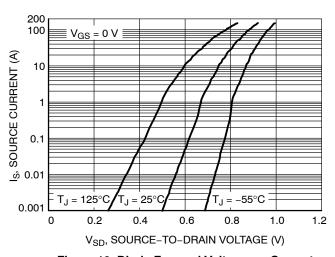
Figure 10. Diode Forward Voltage vs. Current
