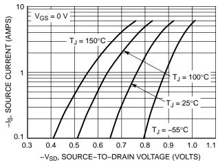
Figure 7. Diode Forward Voltage vs. Current
