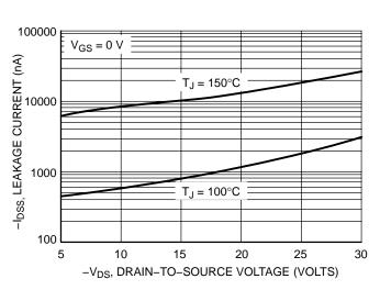
Figure 6. Drain-to-Source Leakage Current vs. Voltage
