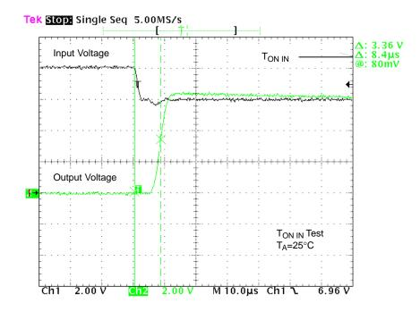
Figure 9. Ton IN Waveforms
