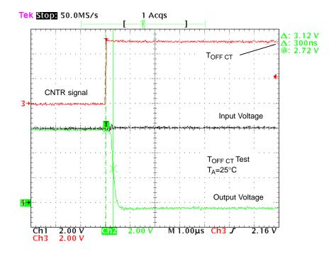
Figure 13.  $T_{OFF\ CT}$  Waveforms
