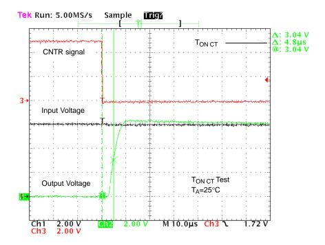
Figure 12. T<sub>ON CT</sub> Waveforms
