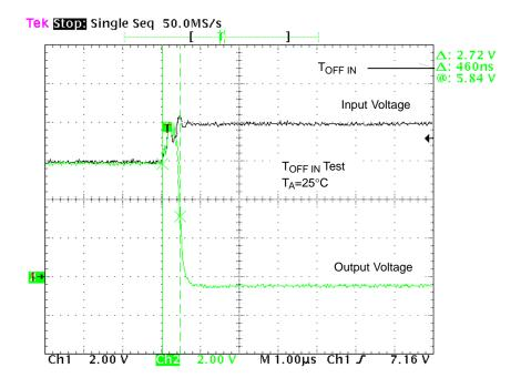
Figure 10. T<sub>OFF IN</sub> Waveforms
