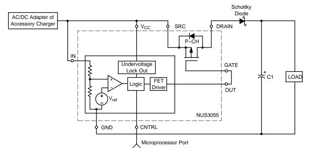
Figure 1. Simplified Schematic
