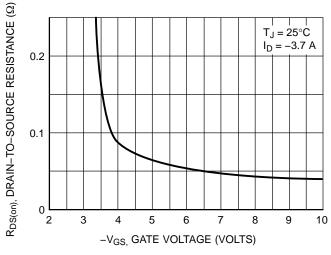
Figure 5. On–Resistance vs. Gate–to–Source Voltage
