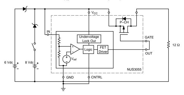
Figure 8. Test Circuit for  $\rm T_{ON\;IN}$  and  $\rm T_{OFF\;IN}$
