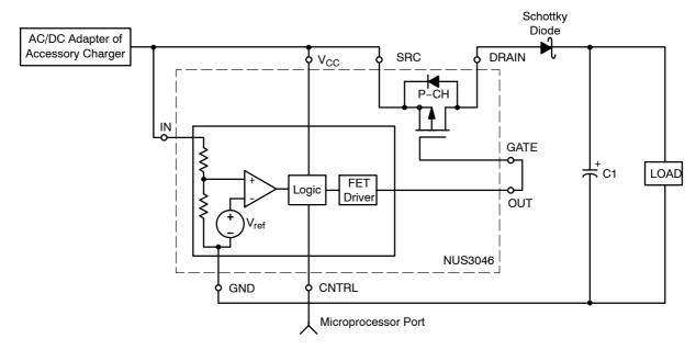
Figure 1. Simplified Schematic
