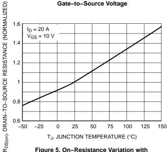
Figure 5. On–Resistance Variation with Temperature
