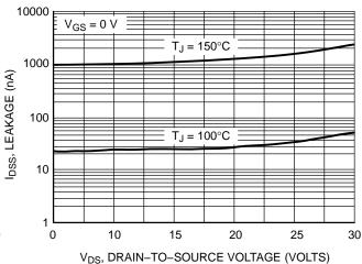
Figure 6. Drain-to-Source Leakage Current versus Voltage
