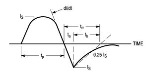
Figure 14. Diode Reverse Recovery Waveform
