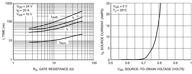
Figure 9. Resistive Switching Time Variations versus Gate Resistance
