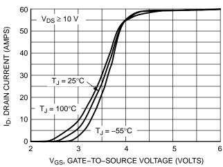
Figure 2. Transfer Characteristics
