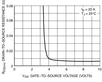
Figure 3. On–Resistance versus Gate–to–Source Voltage
