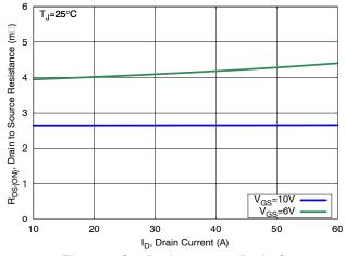
Figure 4. On-Resistance vs. Drain Current
