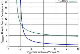
Figure 3. On-Resistance vs. Gate Voltage
