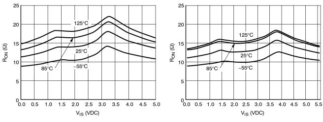
Figure 22. R<sub>ON</sub> vs. Temp,  $V_{CC}$  = 5.0 V
