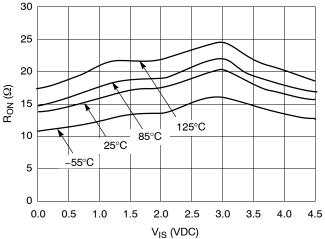
Figure 21.  $R_{ON}$  vs. Temp,  $V_{CC}$  = 4.5 V
