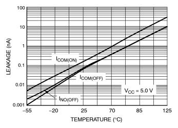
Figure 9. Switch Leakage vs. Temperature
