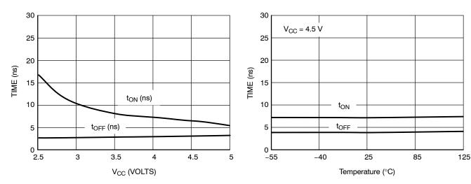
Figure 12.  $t_{ON}$  and  $t_{OFF}$  vs.  $V_{CC}$  at 25  $^\circ C$
