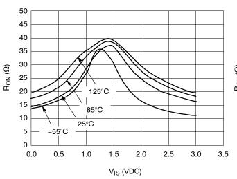
Figure 20. R<sub>ON</sub> vs. Temp,  $V_{CC}$  = 3.0 V
