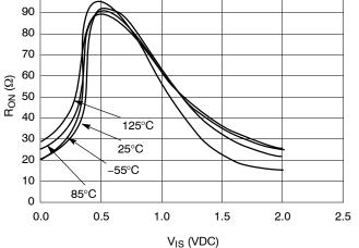
Figure 18. R<sub>ON</sub> vs Temp, V<sub>CC</sub> = 2.0 V
