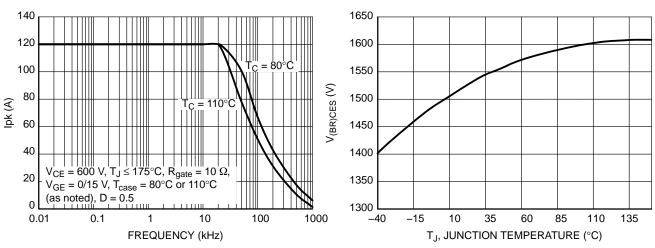
Figure 19. Collector Current vs. Switching Frequency
