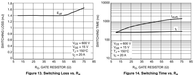
Figure 13. Switching Loss vs. Ra
