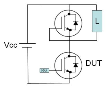
Figure 22. Test Circuit for Switching Characteristics
