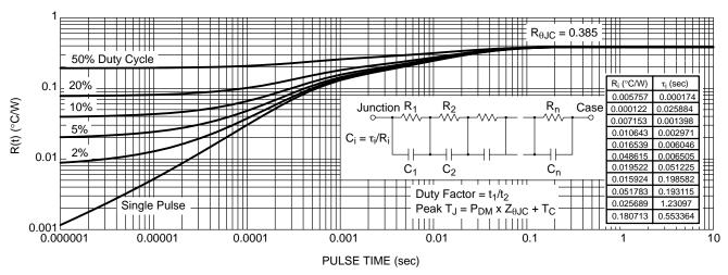
Figure 21. IGBT Transient Thermal Impedance
