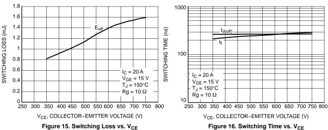
Figure 15. Switching Loss vs. V<sub>CE</sub>
