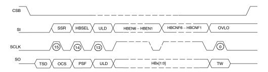
Figure 13. SPI Communication Frame Format
