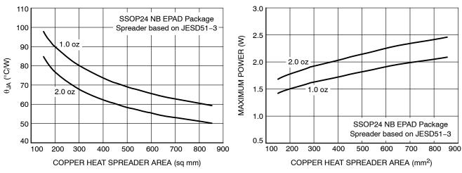
Figure 25.  $\theta_{JA}$  vs. Cu Area: SSOP24 NB EP
