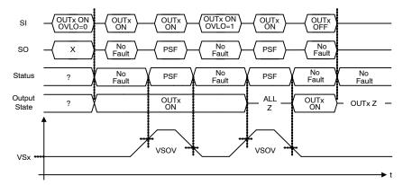
Figure 21. Over-Voltage Timing Diagram
