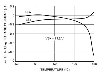
Figure 12. Source-Sink Leakage vs. Temperature
