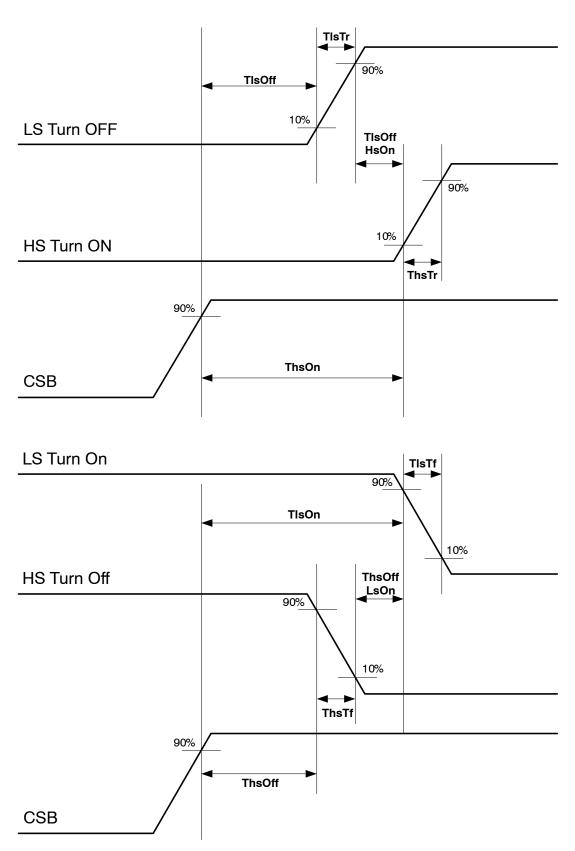
Figure 4. Detailed Driver Timing
