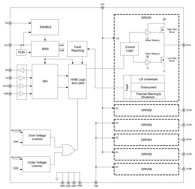
Figure 2. Block Diagram
