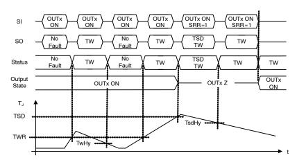
Figure 24. Thermal Warning and Shutdown Timing Diagram
