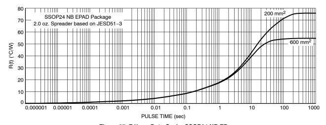
Figure 27. R(t) vs. Duty Cycle: SSOP24 NB EP
