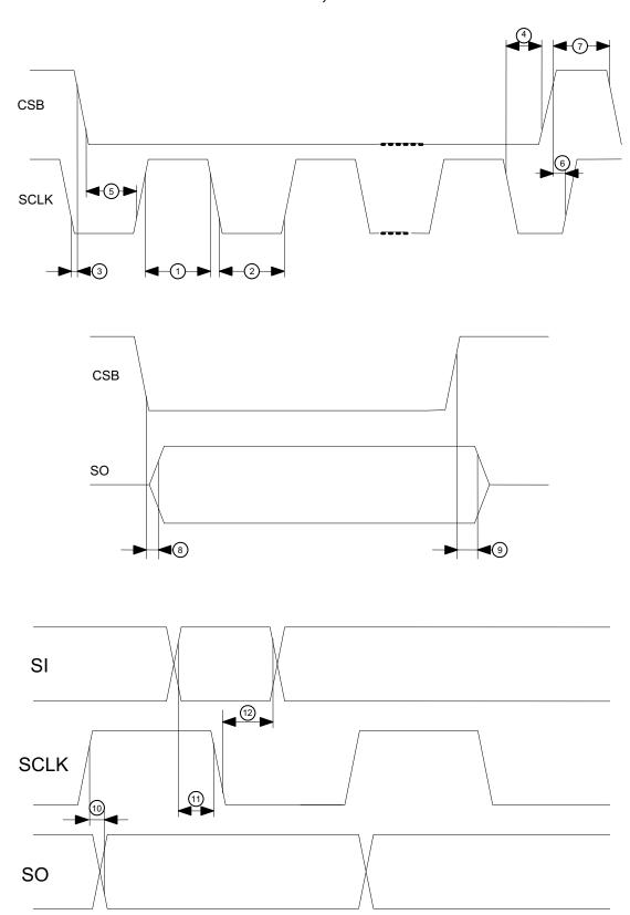
Figure 5. Detailed SPI Timing
