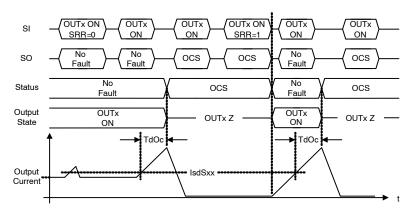
Figure 22. Over-Current Timing Diagram
