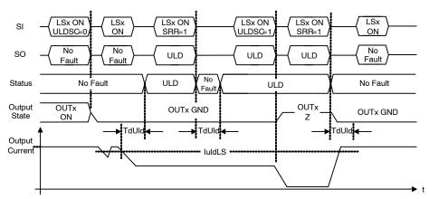
Figure 23. LS Under-load Timing Diagram
