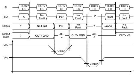
Figure 20. Under-Voltage Timing Diagram
