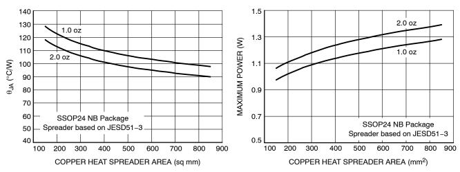
Figure 28.  $\theta_{JA}$  vs. Cu Area: SSOP24 NB
