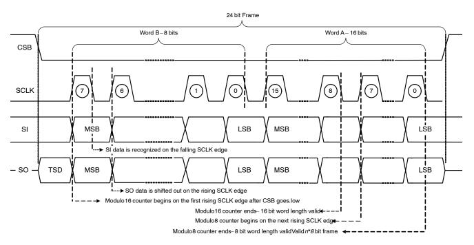
Figure 16. SPI Data Recognition and Frame Detection
