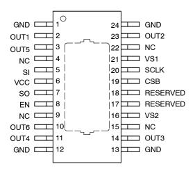
Figure 3. Pinout - SSOP24 NB and SSOP24 NB EP (Top View)
