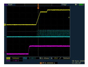
Figure 8. Typical Startup Waveforms
