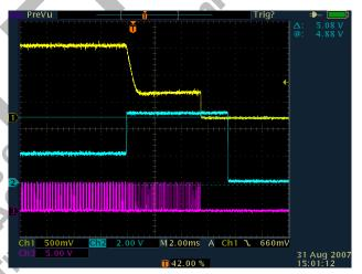
Figure 9. Overcurrent Latchoff Waveforms
