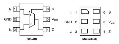
Figure 1. Pinout Diagrams (Top Views)
