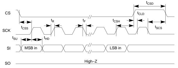
Figure 16. SPI Input Timing
