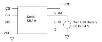
Figure 15. Battery Back-Up Version Schematics
