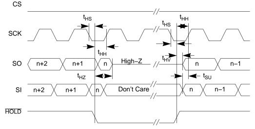
Figure 18. SPI Hold Timing
