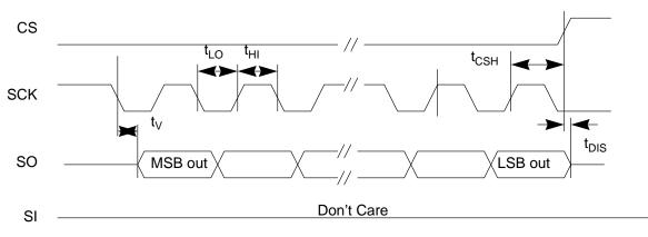
Figure 17. SPI Output Timing
