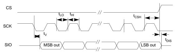
Figure 20. QUAD Output Timing
