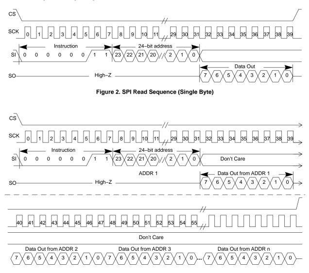
Figure 3. SPI Read Sequence (Sequential Bytes)
