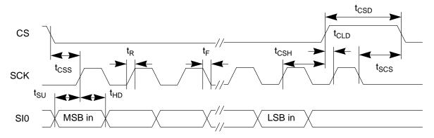
Figure 19. QUAD Input Timing
