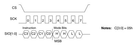
Figure 10. DUAL Read Mode Register Sequence (RDMR)
