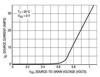
Figure 10. Diode Forward Voltage versus Current
