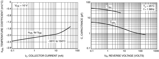
Figure 5. Base-Emitter Temperature Coefficient
