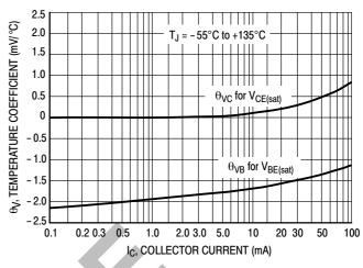
Figure 5. Temperature Coefficients
