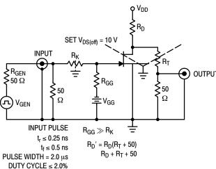
Figure 5. Switching Time Test Circuit
