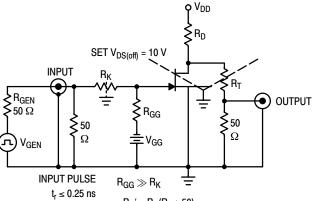
Drain-Source Voltage (VDS) is slightly lower than Drain Supply Voltage (VDD) due to the voltage divider. Thus Reverse Transfer Capacitance (Crss) or Gate-Drain Capacitance (Cgd) is charged to  $V_{GG} + V_{DS}$ .
