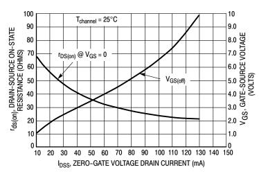
Figure 10. Effect of I<sub>DSS</sub> On Drain-Source Resistance and Gate-Source Voltage
