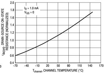
Figure 9. Effect of Temperature On **Drain-Source On-State Resistance**
