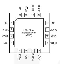
Figure 3. Pin Assignments (Top View)
