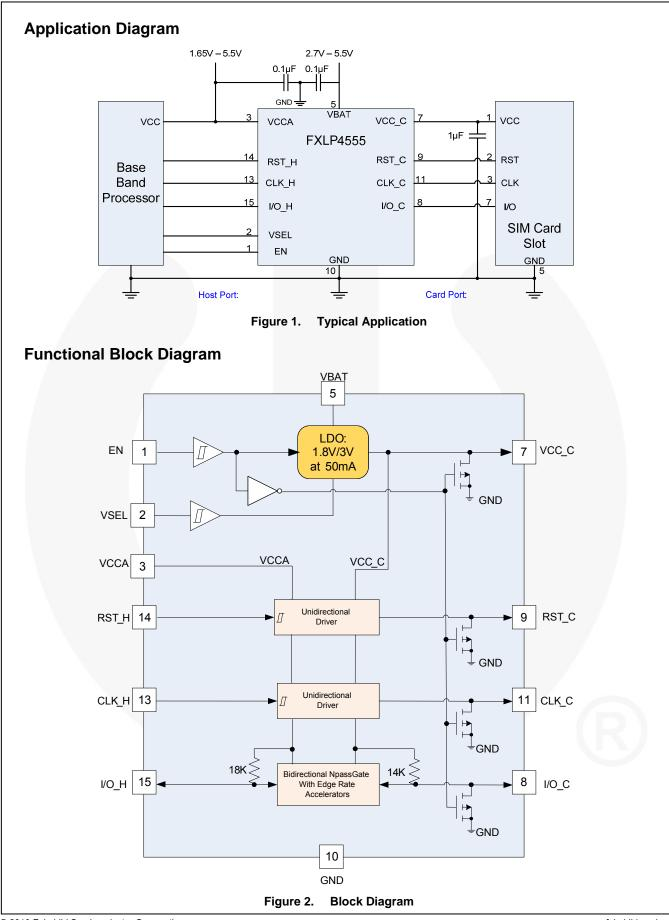
FXLP4555 — 1.8V / 3.0V SIM Card Power Supply and Level Shifter
