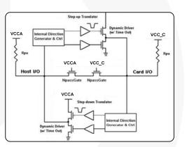
Figure 9. Basic I/O Line Interface
