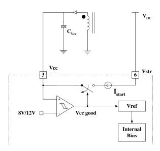
Figure 4. Internal startup circuit
