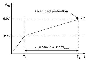
Figure 7. Over Load Protection
