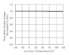
Burst Mode Enable Voltage vs. Temperature
