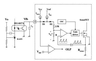
Figure 5. Pulse width modulation (PWM) circuit
