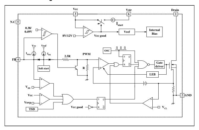
Figure 2. Functional Block Diagram of FSDM1265RB
