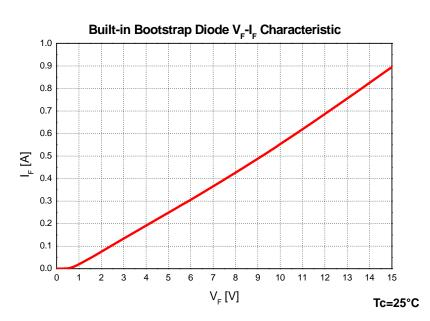
Figure 2. Built-in Bootstrap Diode Characteristics (Typical)
