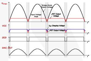
Figure 5. Internal PFC Function
