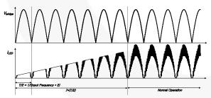
Figure 4. Soft-Start Function in AC Input Mode
