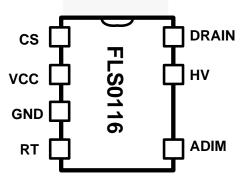
Figure 3. Pin Configuration
