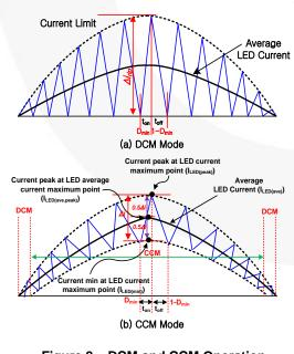
Figure 8. DCM and CCM Operation
