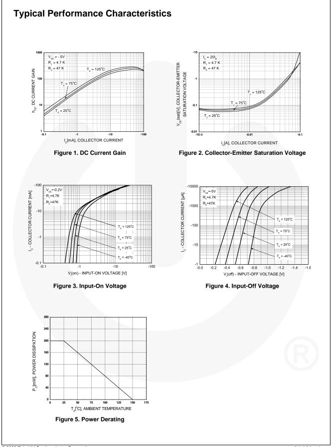
FJV4114R — PNP Epitaxial Silicon Transistor with Bias Resistor
