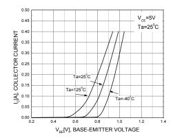
Figure 6. Base-Emitter On Voltage
