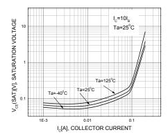
Figure 4. Collector-Emitter Saturation Voltage
