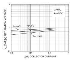
Figure 5. Base-Emitter Saturation Voltage
