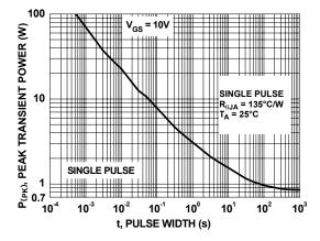
Figure 12. Single Pulse Maximum Power Dissipation
