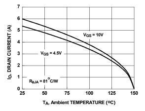
Figure 10. Maximum Continuous Drain Current vs
