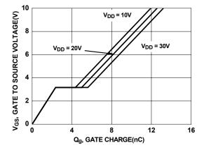
Figure 7. Gate Charge Characteristics
