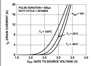
Figure 5. Transfer Characteristics
