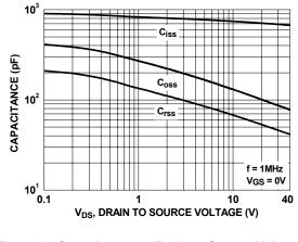
Figure 8. Capacitance vs Drain to Source Voltage
