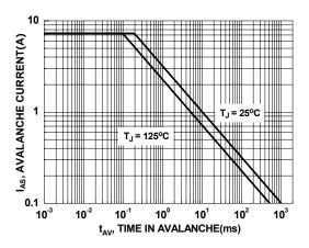
Figure 9. Unclamped Inductive Switching Capability
