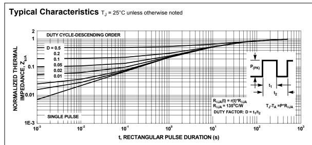
Figure 13. Transient Thermal Response Curve
