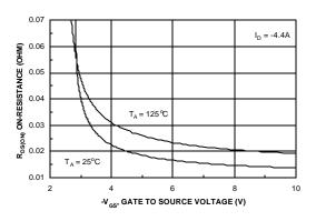
Figure 4. On-Resistance Variation with Gate-to-Source Voltage.
