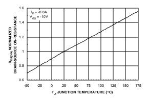
Figure 3. On-Resistance Variation with Temperature.
