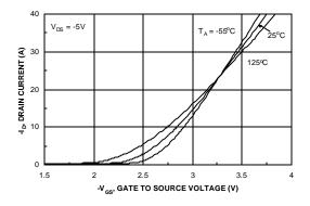
Figure 5. Transfer Characteristics.
