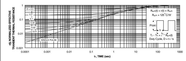
Figure 11. Transient Thermal Response Curve.
