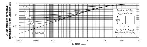
Figure 12. Transient Thermal Response Curve.
