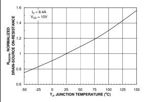
Figure 3. On-Resistance Variation with Temperature.
