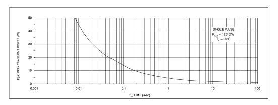
Figure 11. Single Pulse Maximum Power Dissipation.
