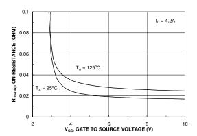
Figure 4. On-Resistance Variation with Gate-to-Source Voltage.
