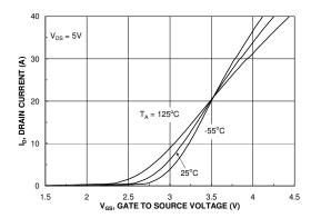
Figure 5. Transfer Characteristics.
