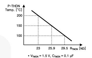
Figure 36. R<sub>TMON</sub> vs. P-THDN Temperature
