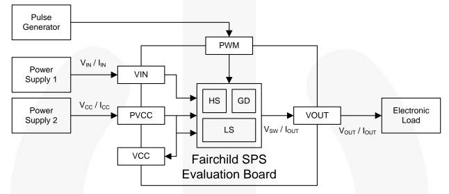
Figure 38. Power Loss and Efficiency Measurement Diagram
