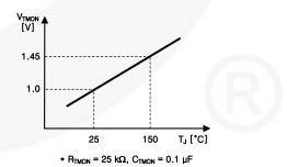
Figure 35. Gate Driver T<sub>J</sub> vs. V<sub>TMON</sub>
