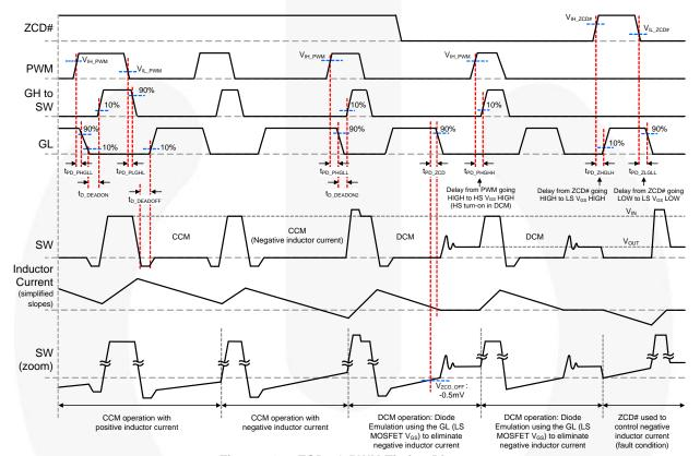
Figure 34. ZCD# & PWM Timing Diagram
