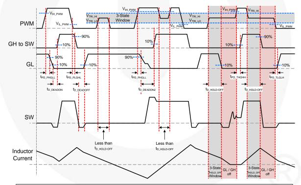
$t_{PD,XXX}$  = propagation delay from external signal (PWM, ZCD#, etc.) to IC generated signal. Example:  $t_{PD,PHGLL}$  - PWM going HIGH to low-side MOSFET  $V_{GS}$  (GL) going LOW  $t_{D,XXX}$  = delay from IC generated signal to IC generated signal. Example:  $t_{D,DEADON}$  - low-side MOSFET  $V_{GS}$  LOW to high-side MOSFET  $V_{GS}$  HIGH
