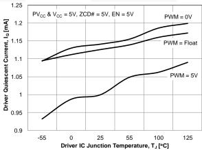
Figure 24. Driver Shutdown Current vs. Temperature
