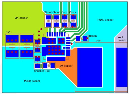
Figure 39. Single-Phase Board Layout Example - Top View
