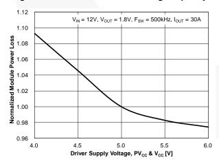
Figure 7. Power Loss vs. Input Voltage
