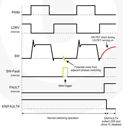
Figure 37. Catastrophic Fault Waveform
