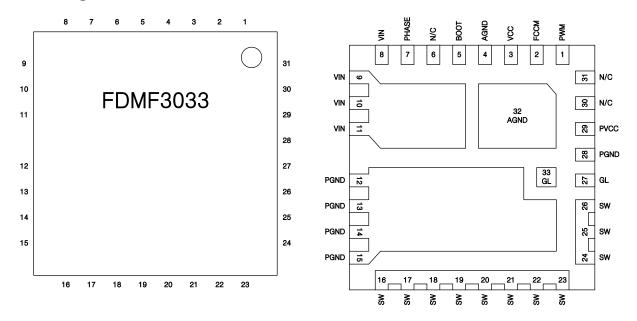
Figure 3. Pin Configuration - Top View and Transparent View
