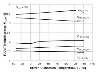
**FCCM Threshold vs. Driver** Figure 19. **Supply Voltage**
