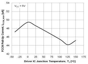
**FCCM Threshold vs. Temperature** Figure 20.
