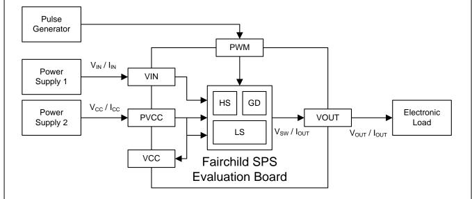
Figure 30. Power Loss and Efficiency Measurement Diagram
