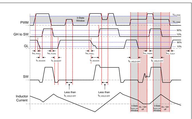
Figure 28. PWM 3-State Timing Diagram (FCCM held HIGH)
