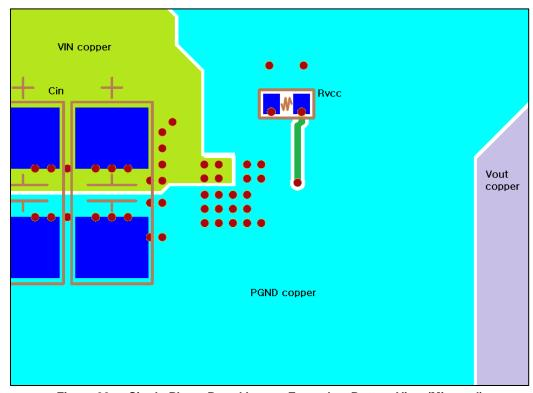
Figure 32. Single-Phase Board Layout Example – Bottom View (Mirrored)
