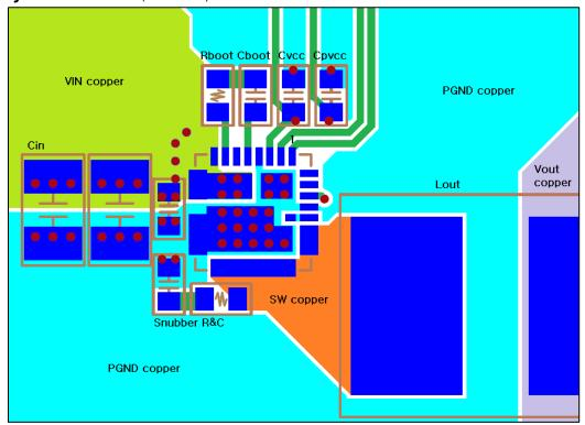
Figure 31. Single-Phase Board Layout Example - Top View
