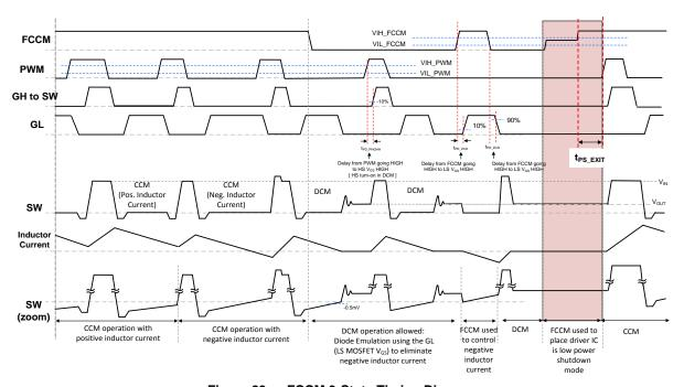
Figure 29. FCCM 3-State Timing Diagram
