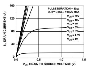
Figure 8. Saturation Characteristics
