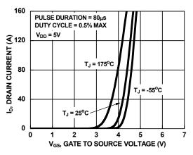
Figure 7. Transfer Characteristics
