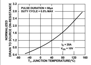
Figure 11. Normalized Rdson vs Junction **Temperature**
