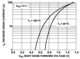
Figure 7. Forward Diode Characteristics
