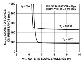
Figure 10. Rdson vs Gate Voltage
