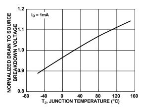
Figure 13. Normalized Drain to Source **Breakdown Voltage vs Junction Temperature**
