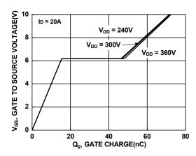
Figure 15. Gate Charge vs Gate to Source Voltage
