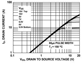
Figure 9. Saturation Characteristics
