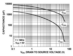
Figure 14. Capacitance vs Drain to Source Voltage
