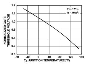
Figure 12. Normalized Gate Threshold Voltage vs **Temperature**
