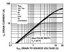
Figure 8. Saturation Characteristics
