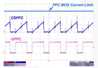
Figure 33. Cycle-by-Cycle Current Limiting
