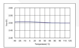
Figure 11. PFC Output Feedback Reference Voltage
