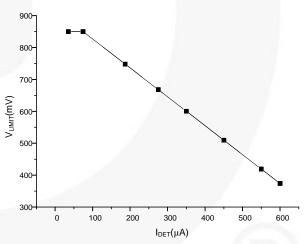
Figure 42. I<sub>DET</sub> Current vs. V<sub>LIMIT</sub> Voltage Characteristic Curve
