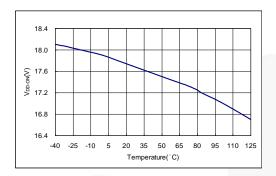
Figure 5. Turn-On Threshold Voltage
