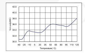
Figure 20. PWM Minimum Off Time for V<sub>FB</sub>=V<sub>G</sub>
