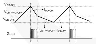
Figure 37. Typical Waveform of V<sub>DD</sub> Voltage and Gate Signal in Hiccup Mode Operation
