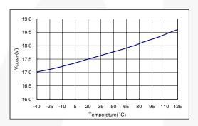
Figure 15. PWM Gate Output Clamping Voltage
