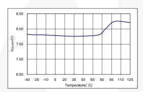
Figure 7. Turn-Off Threshold Voltage
