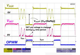
Figure 41. Relationship between  $V_{\text{AUX}}$  and  $V_{\text{IN}}$
