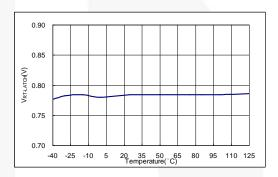
Figure 24. Over-Temperature Protection Threshold Voltage of RT Pin
