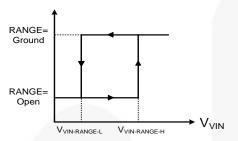
Figure 29. Hysteresis Behavior between RANGE Pin and VIN Pin Voltage
