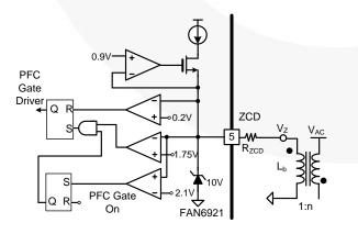
Figure 30. Internal Block of the Zero-Current Detection
