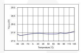
Figure 8. V<sub>DD</sub> Over-Voltage Protection Threshold
