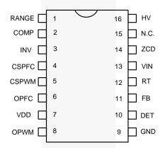
Figure 4. Pin Configuration
