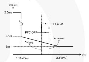
Figure 38. V<sub>FB</sub> Voltage vs. t<sub>OFF-MIN</sub> Time Characteristic Curve
