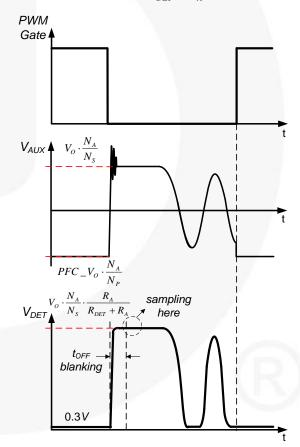
Figure 44. Operation Waveform of Output Over-Voltage Detection
