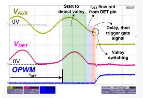
Figure 40. Measured Waveform of Valley Detection
