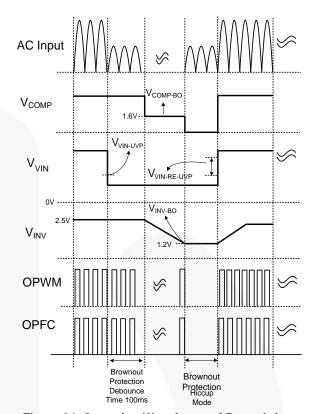
Figure 34. Operation Waveforms of Brownin/out Protection
