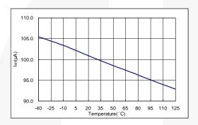
Figure 23. Internal Source Current of RT Pin
