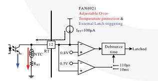
Figure 43. Adjustable Over-Temperature Protection
