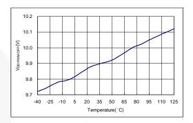
Figure 6. PWM-Off Threshold Voltage
