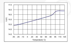
Figure 12. PFC Gate Output Clamping Voltage
