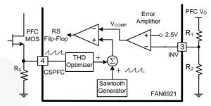
Figure 26. Multi-Vector Error Amplifier with THD Optimizer
