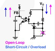
Figure 45. FB Pin Open-Loop, Short Circuit, and Overload Protections
