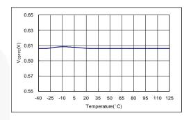
Figure 14. PFC Peak Current Limit Voltage
