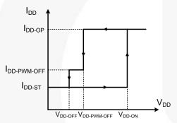
Figure 36. V<sub>DD</sub> vs. I<sub>DD-OP</sub> Characteristic Curve
