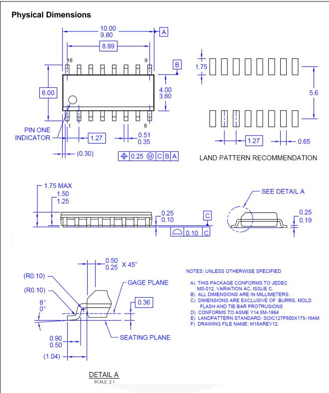
Figure 46. 16-Pin Small Outline Package (SOIC)
