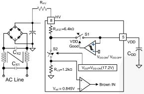
Figure 42. HV Startup Circuit
