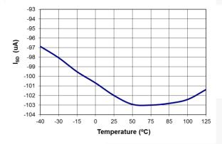
Figure 21. SD Pin Source Current (I<sub>SD</sub>) vs. Temperature
