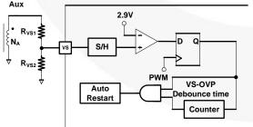
Figure 46. VS-OVP Protection Circuit
