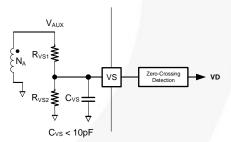
Figure 25. The Valley Detection Circuit
