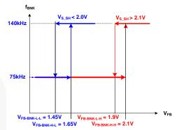
Figure 24. The Blanking Frequency Jumping Point with Variation of V<sub>S-SH</sub>
