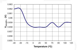
Figure 15. Output Over-Voltage-Protection V<sub>VS-OVP</sub>) vs. Temperature
