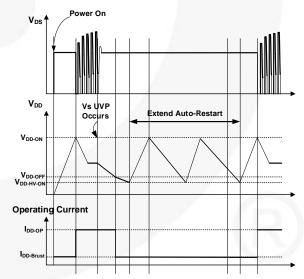
Figure 45. Extend Auto-Restart Mode Operation
