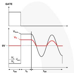
Figure 35. Waveforms for Line Voltage Detection
