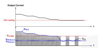
Figure 32. System enter Burst-Mode Behavior
