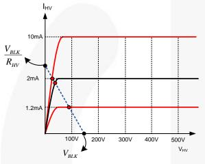
Figure 43. Characteristics of HV pin
