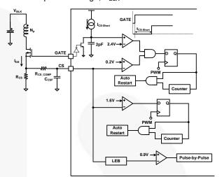
Figure 49. Current Sense Protection Circuit
