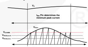
Figure 31. Burst-Mode Operation with IMIN
