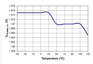
Figure 11. Frequency Jumping point (V<sub>FB-BNK-H-H</sub>) vs. Temperature
