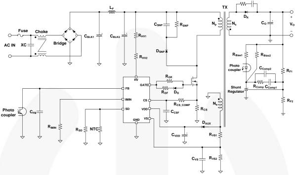
Figure 1. FAN602F Typical Application
