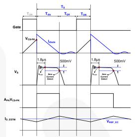
Figure 38. Waveforms for Estimate Output
