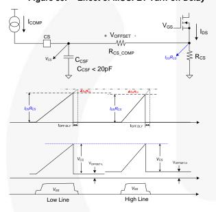
Figure 40. Line Voltage Compensation
