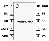
Figure 4. Pin Assignment
