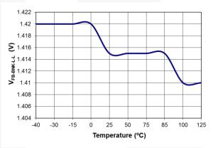
Figure 13. Frequency Jumping point (V<sub>FB-BNK-H-L</sub>) vs. Temperature
