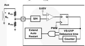
Figure 47. VS-UVP Protection Circuit
