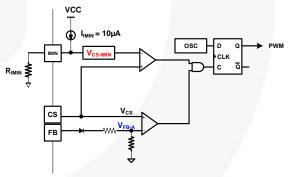
Figure 30. IMIN Function Circuit
