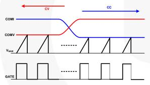
Figure 37. PWM Operation for CV/CC Regulation
