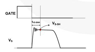
Figure 29. Output Voltage Detection
