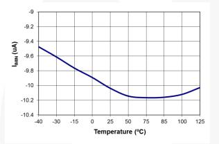
Figure 19. IMIN Pin Current (I<sub>IMIN</sub>) vs. Temperature
