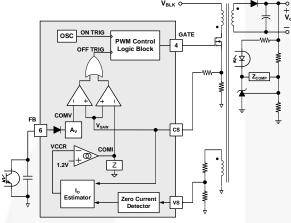
Figure 36. Simplified PWM Control Circuit
