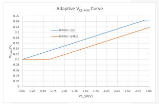
Figure 33. V<sub>CS-IMIN</sub> as a Function of R<sub>IMIN</sub> with Variation of V<sub>S-SH</sub>
