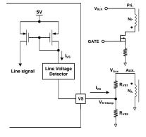
Figure 34. Line Voltage Detection Circuit
