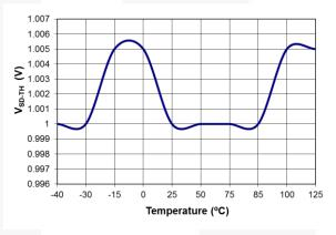
Figure 20. Threshold Voltage for Shutdown Function Enable (V<sub>SD-TH</sub>) vs. Temperature
