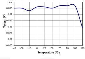
Figure 18. Current Limit Threshold Voltage (V<sub>CS-LIM</sub>) vs. Temperature
