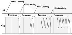
Figure 23. Two Step Blanking Frequency
