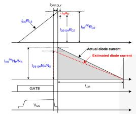
Figure 39. Effect of MOSFET Turn-off Delay
