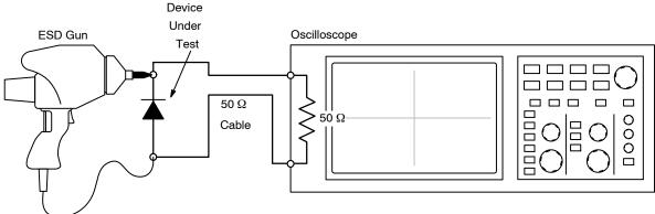
Figure 4. Diagram of ESD Test Setup
