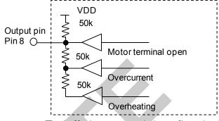
(The buffer has an open drain configuration.)
