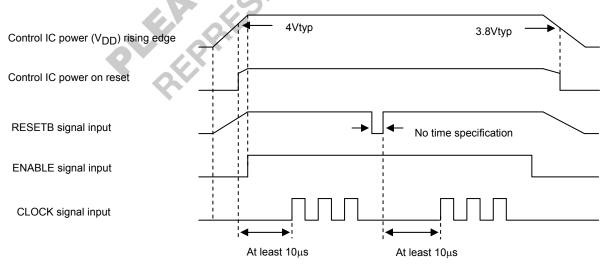
ENABLE, CLOCK, and RESETB Signals Input Timing
