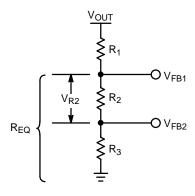
Figure 13. Feedback Sense Resistor Divider Connected Between V<sub>OUT</sub> and Ground
