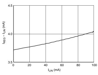
Figure 2. 5.0 V Regulator Bias Current vs. Load Current
