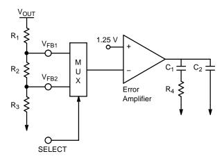
Figure 14. RC Network Used to Compensate the Error Amplifier (OTA)
