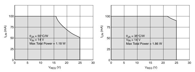
Figure 17. The Shaded Area Shows the Safe Operating Area of the CS5112 as a Function of  $I_{LIN}$ ,  $V_{REG}$ , and  $\theta_{JA}$ . Refer to Table 1 for Typical Loads and Voltages.
