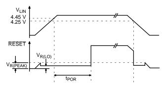
Figure 9. The Power On Reset Time Interval (t<sub>POR</sub>) Begins When V<sub>LIN</sub> Rises Above 4.45 V (Typical)
