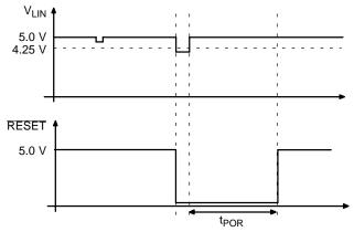
Figure 10. RESET Signal Is Issued Whenever V<sub>LIN</sub> Falls Below 4.25 V (Typical)
