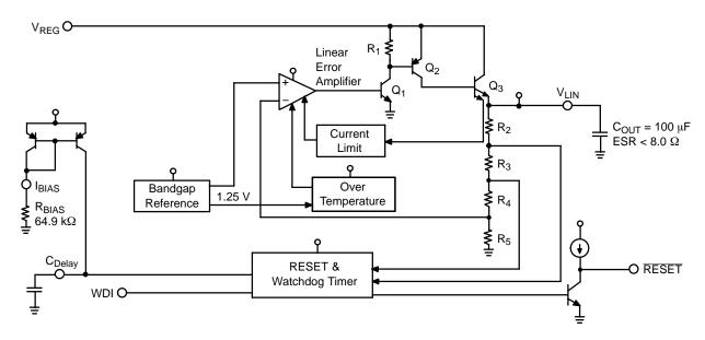
Figure 6. Block Diagram of 5.0 V Linear Regulator Portion of the CS5112
