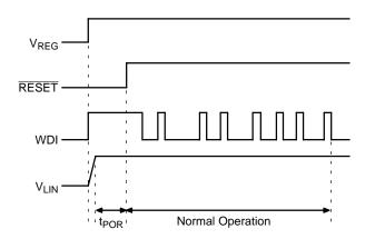
Figure 7. Timing Diagram for Normal Regulator Operation
