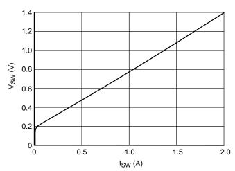
Figure 4. Switch Saturation Voltage
