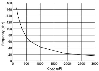
Figure 5. Oscillator Frequency (kHz) vs.  $C_{OSC}$  (pF), Assuming  $R_{BIAS}$  = 64.9  $k\Omega$
