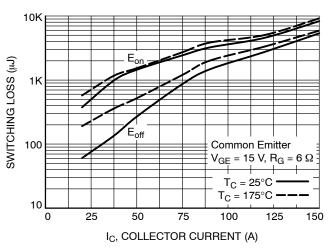
Figure 14. Switching Loss vs. Collector Current
