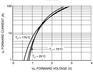
Figure 16. Forward Characteristics
