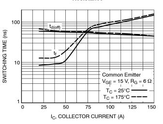
Figure 12. Turn-off Characteristics vs. Collector Current
