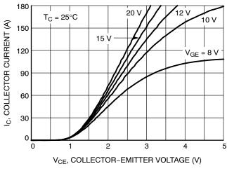
Figure 1. Typical Output Characteristics (25°C)
