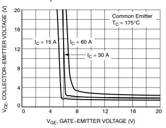
Figure 6. Saturation Voltage vs. V<sub>GE</sub> (175°C)
