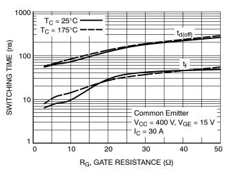
Figure 10. Turn-off Characteristics vs. Gate Resistance
