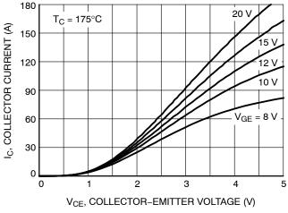
Figure 2. Typical Output Characteristics (175°C)
