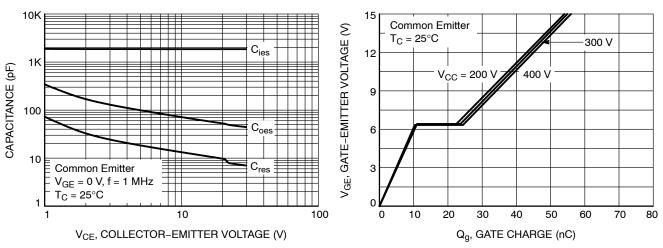
Figure 7. Capacitance Characteristics
