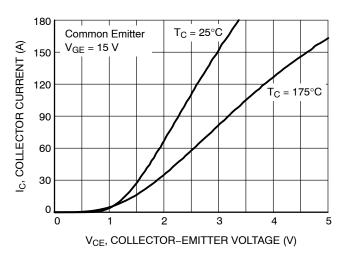
Figure 3. Typical Saturation Voltage Characteristics
