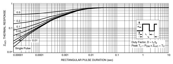
Figure 20. Transient Thermal Impedance of IGBT
