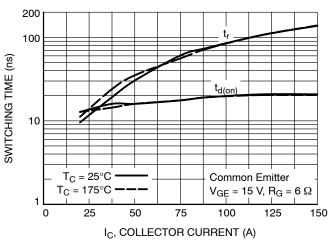
Figure 11. Turn-on Characteristics vs.
