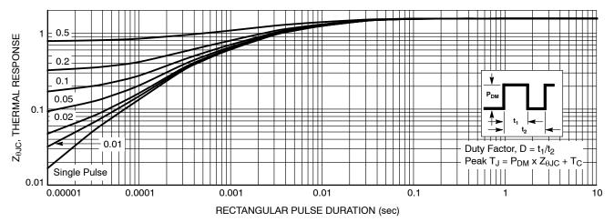
Figure 21. Transient Thermal Impedance of Diode
