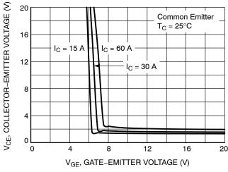
Figure 5. Saturation Voltage vs. V<sub>GE</sub> (25°C)
