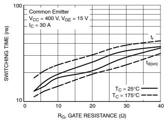
Figure 9. Turn-on Characteristics vs. Gate
