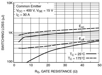
Figure 13. Switching Loss vs. Gate Resistance
