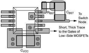
Figure 19. External Component Placement Example
