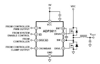
Figure 2. MSOP-10 Package Application Circuit
