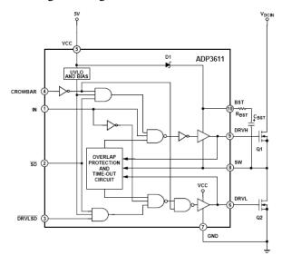
Figure 18. Detailed Block Diagram of the ADP3611
