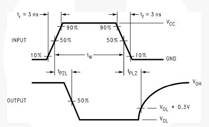
Figure 10. **AC Waveforms**
