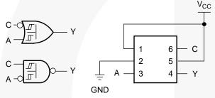
2-Input OR Gate with One Inverted Figure 4. Input 2-Input NAND Gate with One Inverted Input
