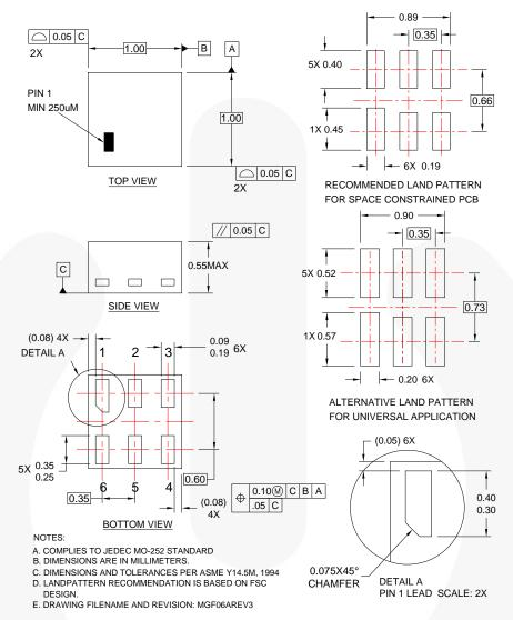
Figure 12. 6-Lead, MicroPak2™, 1x1 mm Body, .35 mm Pitch
