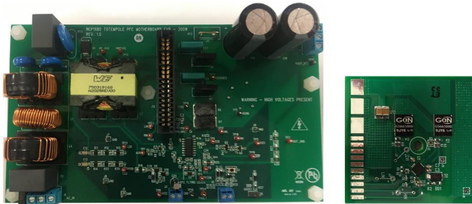
Figure 3. NCP1680 Evaluation Board along with a Daughter Card Featuring Fast Leg Switches
