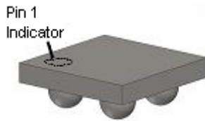
Figure 3. WLCSP Bumps Facing Down (Top View)
