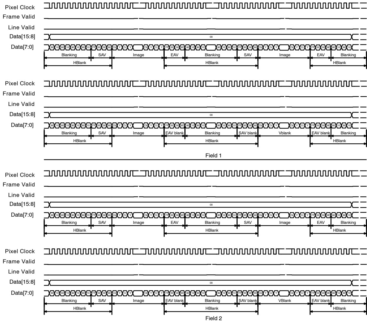
Figure 18. Typical CCIR656 Output
