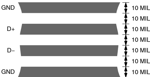
Figure 19. Arrangement of Signal Tracks
