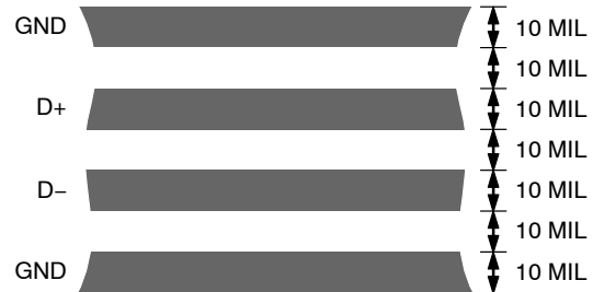
Figure 18. Arrangement of Signal Tracks
