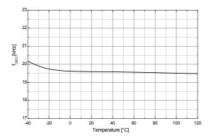
Figure 23. Operating Frequency 1 vs. Temperature
