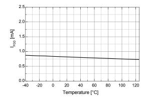
Figure 18. I<sub>PDD</sub> vs. Temperature
