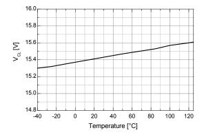
Figure 16.  $V_{BS}$  UVLO- vs. Temperature
