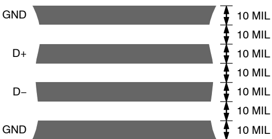
Figure 15. Arrangement of Signal Tracks
